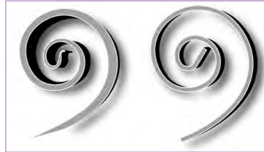
The scroll on the far left is made of stock that has been drawn to a taper and bent hot, free-hand. On the right is a scroll made of stock section, bent cold, with a typically straight centre where it was clamped to a scroll-forming jig.
