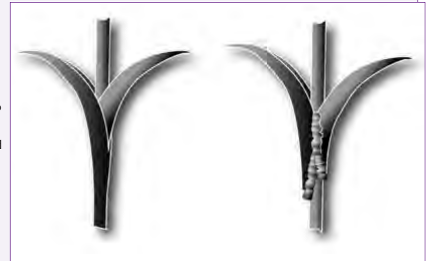
Right, leaf detail fire-welded to a round bar. Far right, leaf detail arc welded to a round bar.
