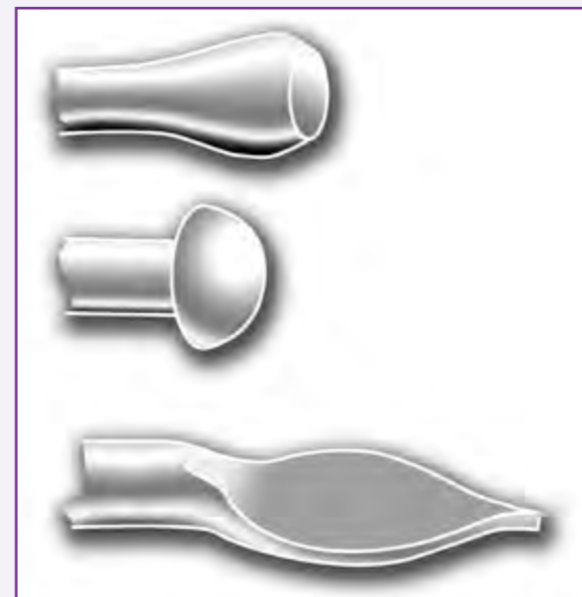
Top, bar-end, thickened by upsetting. Middle, bar-end, upset and formed into rivet head. Bottom, bar-end, upset and formed into finial.
