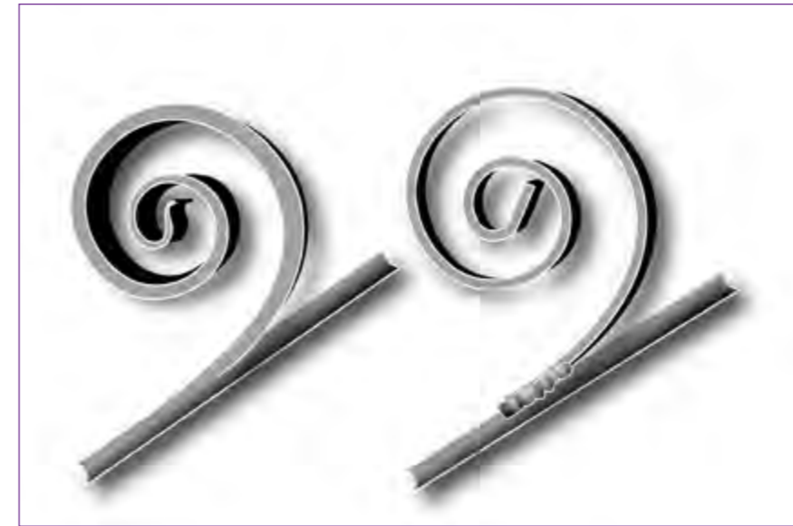
Far left, forged scroll fire-welded to a round bar. Right, cold-bent scroll arc welded to a round bar.
